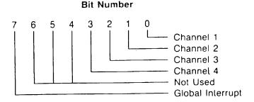
Under compatible mode, (since COM1: and COM2: are handled by PC system) bit 0 and bit 1 of interrupt vector are not used.
